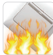
850° C Glow wire test, flame dieoff within 30 seconds.
